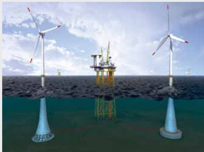
Offshore windmill foundations. Image courtesy Olav Olsen
