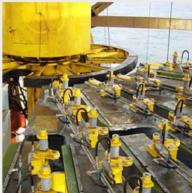
Fingerboard with latches Image courtesy Aanestad Engineering
